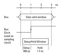
(The actual sampling position is in the middle of the setup/hold window.)
