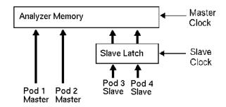
When the slave clock occurs, data captured on the pods that use the slave clock is saved in a slave latch. Then, when the master clock occurs, data captured on the pods that use the master clock, as well as the slave latch data, are saved into logic analyzer memory.
