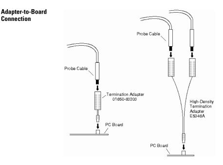
Both the 01650-63203 and the E5346A adapters include termination for the logic analyzer. The 01650-63203 termination adapter plugs into a 2 x 10 pin header with 0.1 inch spacing. The E5346A high-density adapter connects to an AMP "Mictor 38" connector. If possible, use support shrouds around the Mictor connector to relieve strain and improve connections.
