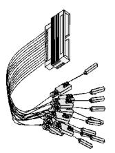
The standard lead set plugs directly into any .1-inch grid with 0.026 to 0.033-inch diameter round pins or 0.025-inch square pins. All probe tips work with the Agilent Technologies 5059-4356 surface mount grabbers and the Agilent Technologies 5959-0288 through-hole grabbers.
